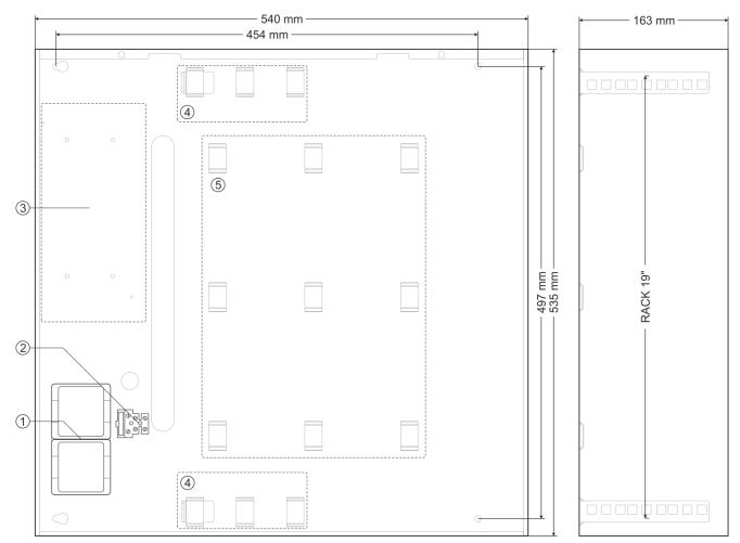
Fig. 1. The enclosure view
